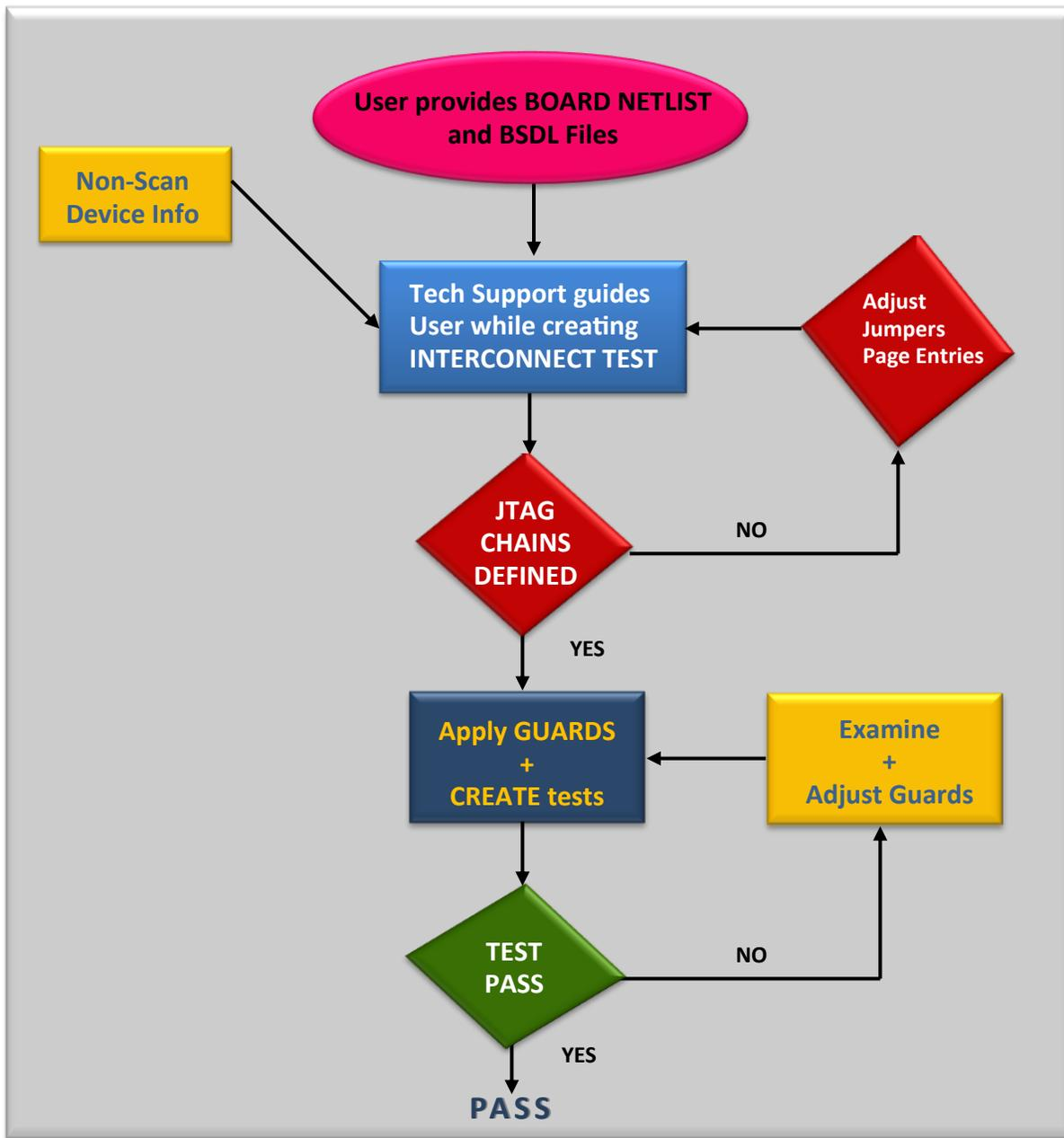
*The onTAP Boundary Scan TEST DEVELOPMENT and DEBUG process. Flynn Systems' Tech Support can interactively assist to quickly achieve passing tests.*
